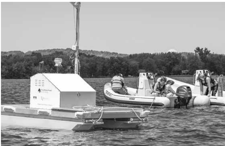
DAVE MUNCH / PHOTO EDITOR Jefferson Project team members, from left, Nina Bellus, Amanda Kelly, Amanda Matkosky and Kate Audino work to anchor a vertical profiler into its final position on Chautauqua Lake on June 23. The two profilers — one each placed in the lake’s north and south basins — track water conditions from the surface to the bottom, quantify water circulation patterns and monitor local weather conditions.
