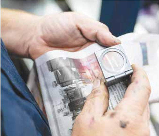
Griffis uses a magnifying glass to check that each of four color printing plates are aligned.
