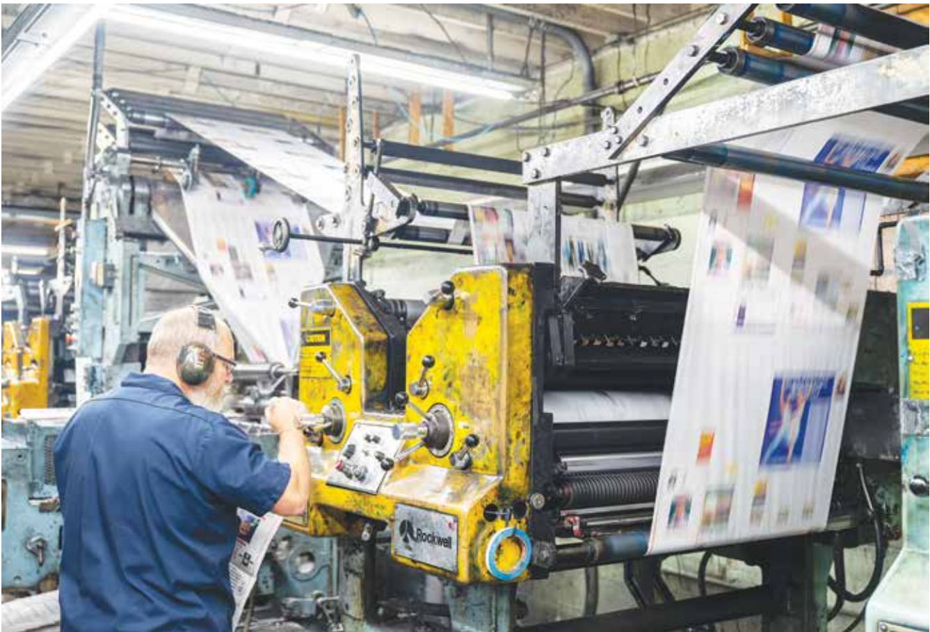
Griffis adjusts the press to ensure each of four color printing plates are in alignment. The alignment of the plates, known as registration, is critical for images to print clearly.
